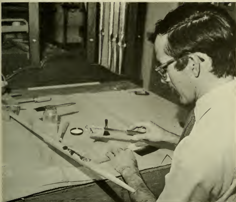
Conservator Scott Odell applies gold leaf over gesso to front pipes for restoration of chamber organ by John Snetzler, London, 1761.
