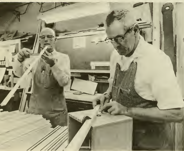
Exhibits fabricators Herbert L. Brumback (left) and Olaf L. Leatherland construct coin cabinets for the Lilly Collection. Utmost accuracy of measurement was required to insure the necessary tight seal (photo courtesy Larry Stevens).
